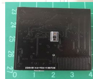
Smart Board Bottom View - Location of the Heart rate sensor
