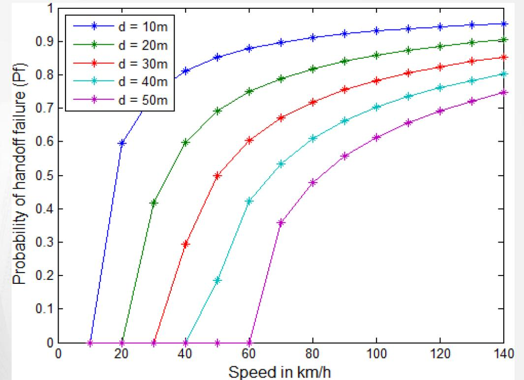
**Figure 6:** Relationship between probability of handover failure and speed for angle  $\theta_1$  (more than 30 degree) and with handover signaling delay of 3 s
