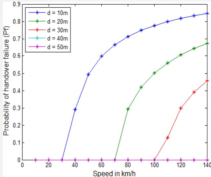
**Figure 3:** Relationship between probability of handover failure and speed for angle  $\theta_1$  (less than 30 degree) with handover signaling delay of 1 s
