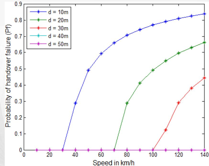
**Figure 4:** Relationship between probability of handover failure and speed for angle  $\theta_1$  (more than 30 degree) and with handover signaling delay of 1 s
