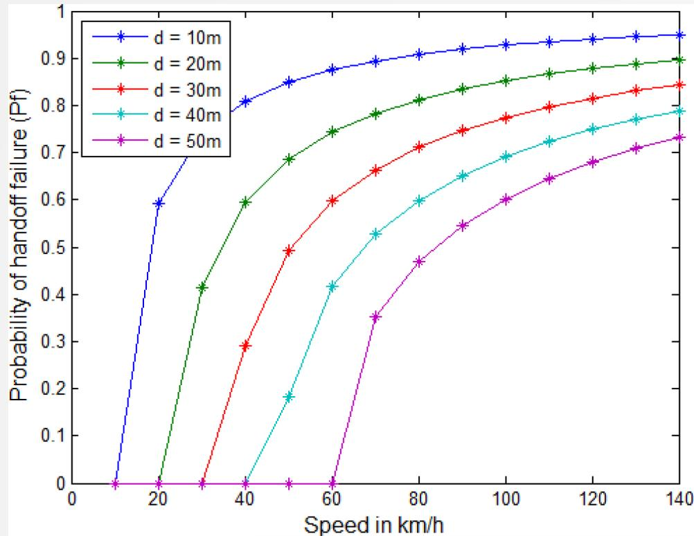
**Figure 5:** Relationship between probability of handover failure and speed for angle  $\theta_1$  (less than 30 degree) and with handover signaling delay of 3 s
