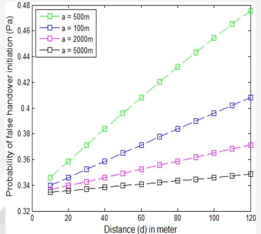
Figure 2: Relationship between false handover initiation probability and distance
